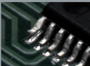
Lifted lead, angled view
