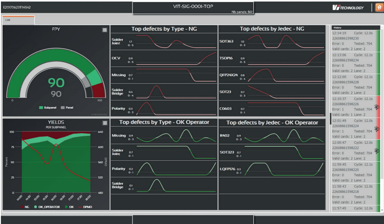
"First-pass yield is improving but two issues are revealed by trend charts: bad component reference loaded in placement machine (OCV) and unstable polarity check on LQFP176 component."
