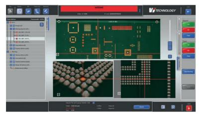
**PI Series:** PI's patented Z-referencing method leverages the entire textured 3D board information, rather than just cropped images around the pads, to define a stable and accurate Z-reference.
