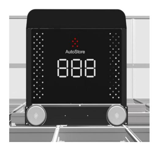
B1 Robots have 75% higher acceleration compared to R5 Robots, enabled by direct drives in each driving wheel.
